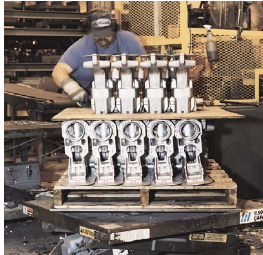
Combination lift & turntable to build up and/or break down pallets of casting
