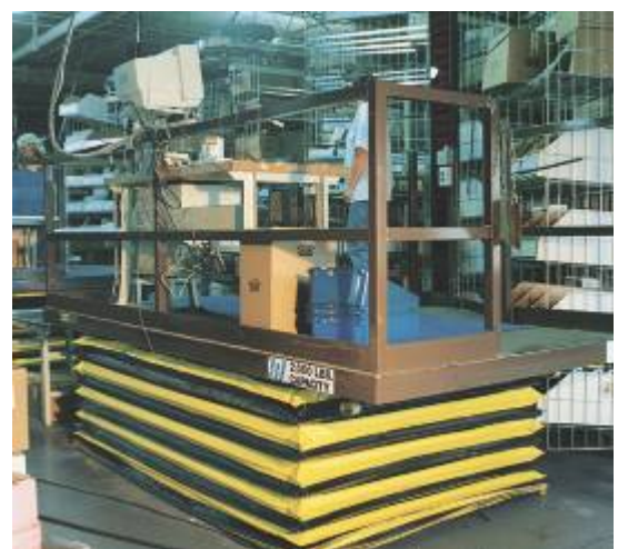
Lift bringing the worker to the work in a parts-pulling application
